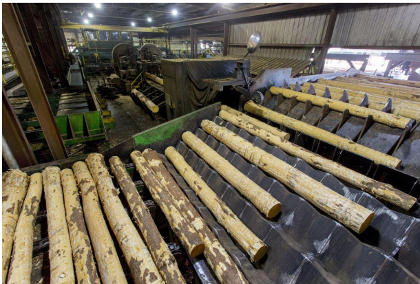
Pine logs move along as a computer decides what size lumber they will become. PHOTO: KAREN E. SEGRAVE FOR THE WALL STREET JOURNAL
